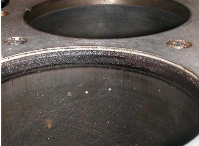
This is a failed gasket – hard to tell the difference until the heads come off
