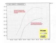
The graph illustrates the power curves before and after a "stage 1" upgrade
