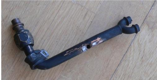
And while we are at it, attempting to repair the damaged pipe yourself might not be a terribly good idea. R134a air conditioning gas is pressurised to 300PSI and if your repair fails, it will cost another \$200+ for yet another drier and gas refill.
