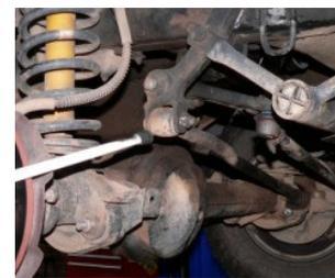
**Worn suspension bushes** will certainly affect the handling of the vehicle, though not always creating vibration in the steering. More likely, the result will be thumps, bangs and the tendency for the vehicle to wander off-line. There are several components that may affect the suspension:
