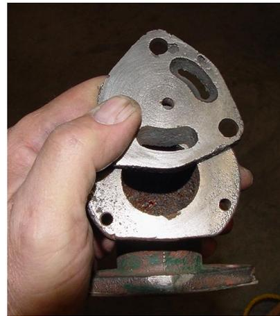
The left picture clearly shows failure through metal fatigue, caused by the bolt being stressed under load. The right hand picture is an example of a porous casting, the voids being caused by bad manufacturing. It is noteworthy that not only metals can be affected by fatigue, with plastic and rubber components being high on the "suspect" list.
